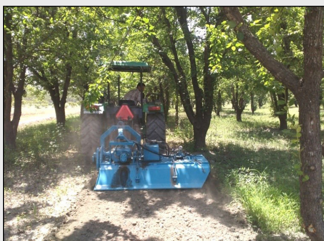
Working of the developed Offset Rotavator in pears orchard
